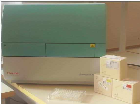
IMAGE 2. The instrument, reagents (PPP reagent, thrombin calibrator, FluCa) and plates used. (Photo by professor Tomas L Lindahl.)
